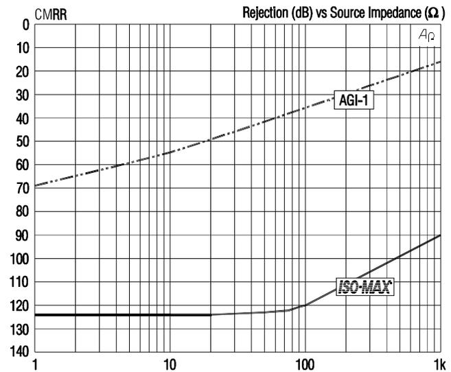
Figure 4 - HUM REJECTION vs SOURCE IMPEDANCE
