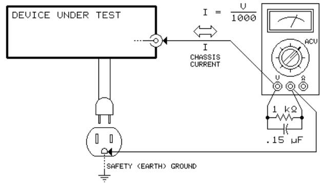
Figure 3 - MEASURING THE CHASSIS CURRENT
